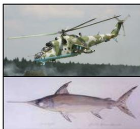
offering three stations, in addition to providing **lift**. The load-out mix is mission dependent; Mi-24s can be tasked with close air support, anti-tank operations, or aerial combat. The body is heavily armored and the **titanium** rotor blades can resist impacts from **.50 caliber** (12.7 mm) rounds. The cockpit is **overpressurized** to protect the crew in **NBC conditions**. See [Wikipedia](#)
